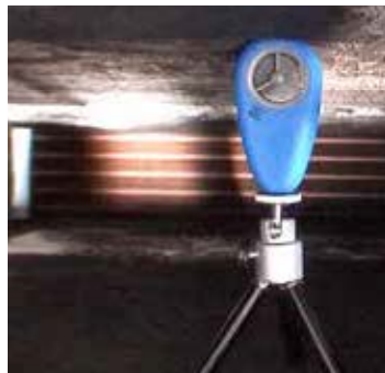
Recording of Ambient Conditions in mixing plenum
